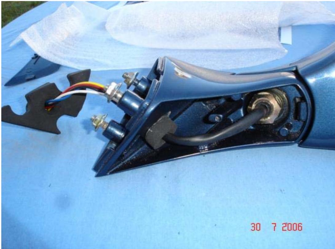
The cable loom can now be carefully withdrawn and pulled out of the hinge spigot.
