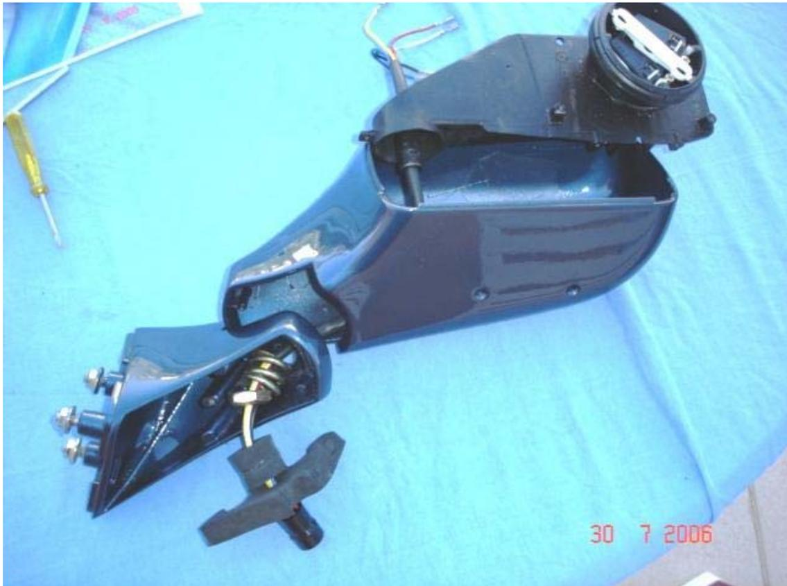
Reassembly is a straight reversal of the above, except for the mirror itself. First engage the spring wires before pressing the mirror back onto its motor.
