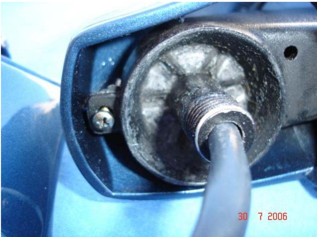
Undo the large nut holding the mirror hinge together (22mm AF). I found that a pipe wrench worked better here than a spanner.
